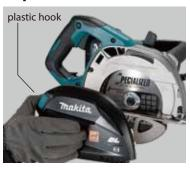
using a mechanism which allows for attaching/detaching simply by one-hand operation of a plastic lever.
