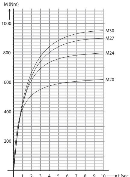
Tightening always depends on the type and the character of the parts to be tightened. Tightening time longer than 10 s only slightly increases the tightening torque.
